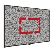
Pixel Shifting is designed to be activated inside the SoC in order to prevent for potential risk of image sticking, caused by constant content. With this feature turned on, pixels on the screen will move in an interval while causing no interference of visual experience.
